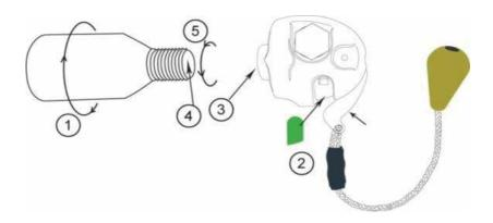
Step 1: Unscrew used CO<sub>2</sub> cylinder in a counterclockwise direction and immediately discard.
