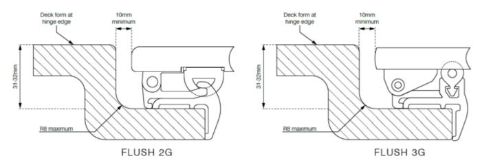
It is essential that the lower frame is placed square on the deck opening. The operation of the hatch should be checked before sealing and fastening to the deck. Each installation should allow for either drainage channels or tube around the hatch to ensure no excess water can become trapped.
