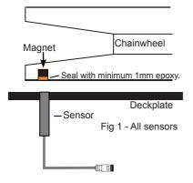
**Note:** If it is not possible to align the sensor and magnet exactly the AA grey sensor may be fitted up to 20mm out of alignment. The AA black sensor and the reed switch sensor must be directly aligned.
