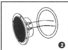
Connect the speaker wires to the speaker.
