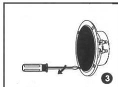
Screw down each of the four Phillips head screws. The locking tabs will swivel into place and secure the unit to the rear surface of the drywall. Put in the strips of adhesive to secure the grille.
