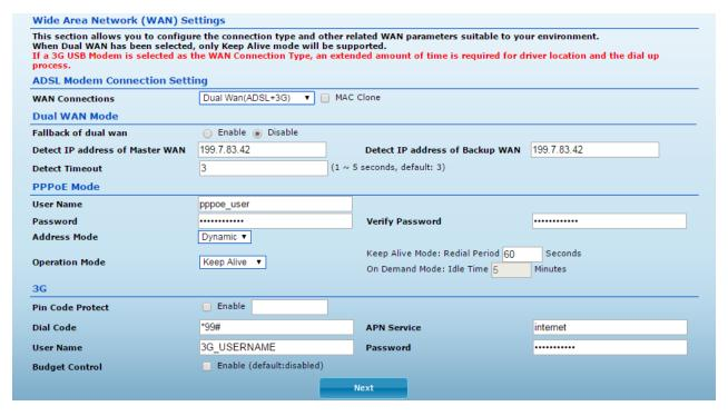
Please refer to Connection type: 3G dongle for setup detail on 3G modem.
