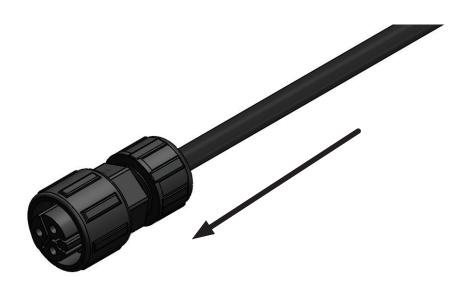
9. Fit and tighten the strain relief and gland nut onto the connector. Plug into the hub, taking care to orient the key correctly. Tighten the cap to make the waterproof seal.
