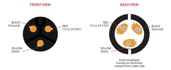
Note: Check the wiring is correct before connecting to the hub. Incorrect wiring can damage the light.
