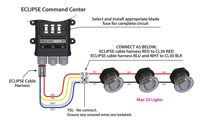
Note : Single color and dual color lights should not be added to the same zone output. Use a separate zone output for each type.
