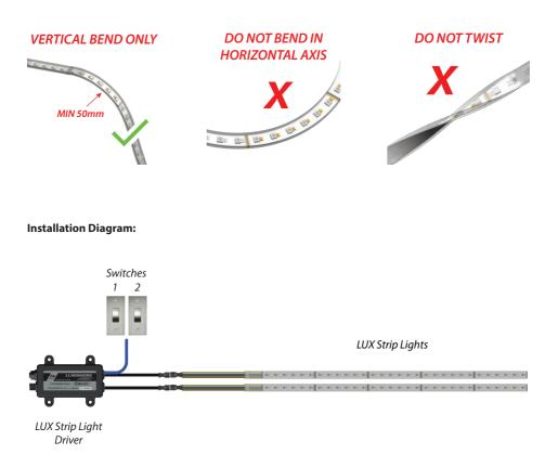
NOTE : The Lumishore Lux Strip Lights requires connection to the Lumishore LUX Strip Light Driver Module. For full electrical installation and wiring diagrams please refer to the LUX Strip Light Driver Installation Manual (45-0143).
