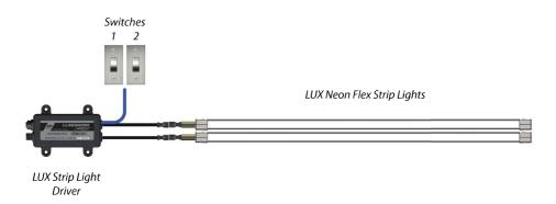
NOTE: The Lumishore LUX Neon Flex Strip Lights requires connection to the Lumishore LUX Strip Light Driver Module. For full electrical installation and wiring diagrams please refer to the LUX Strip Light Driver Installation Manual (45-0143).
