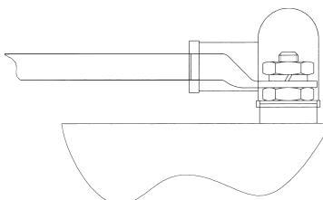
The motor's terminals have no pre-defined polarity. The positive and negative leads may be connected to either terminal.
