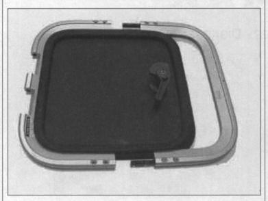
1.7) The seal is stretched over the Acrylic but may have been glued in place to aid assembly. If the seal is removed from the acrylic the acrylic will need cleaning, solvents should not be used
