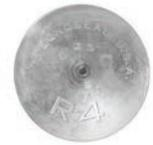
R4 anodes included to prevent electrolysis damage
