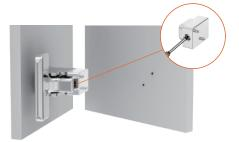
Swing door closed to mark installation holes for strike plate. Then, use a screwdriver through side openings to easily remove marking punch.
