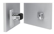
Reinsert rubber bumper and install the strike plate on opposing surface using markings from previous step.
